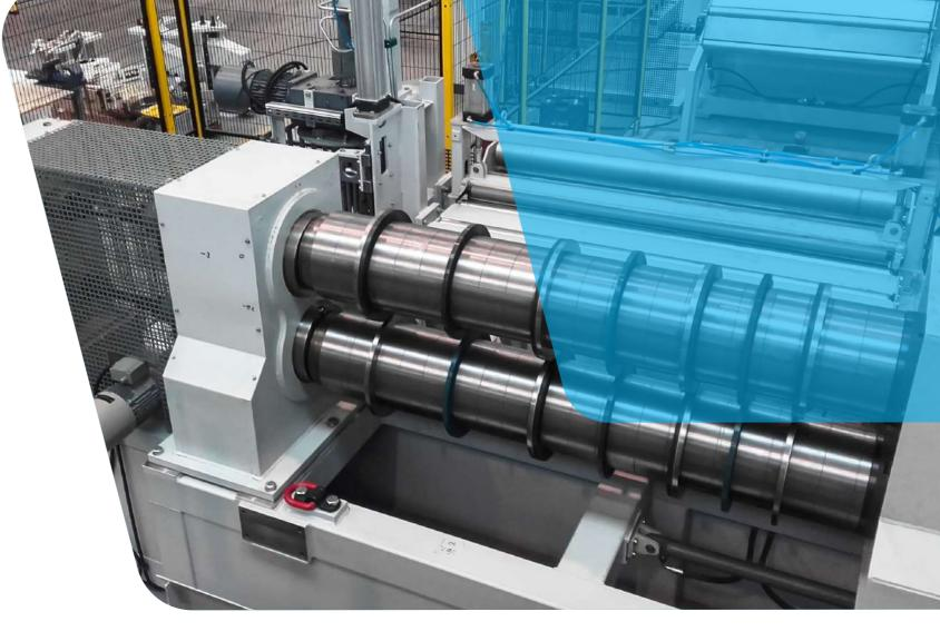
Optionally, it is possible to equip the shears with a quick-change system for circular knives, recommended if you need to make frequent changes in the cutting process.
